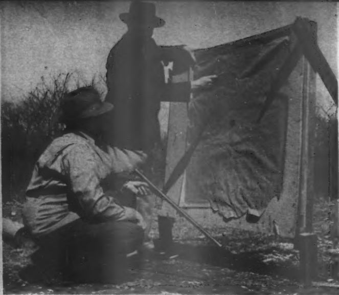
This pattern board is a wooden frame with composition backing onto which is tacked wrapping paper with an aiming mark in the center. Patterning not only shows the shooter where his gun is shooting but what sort of pellet distribution he is getting
